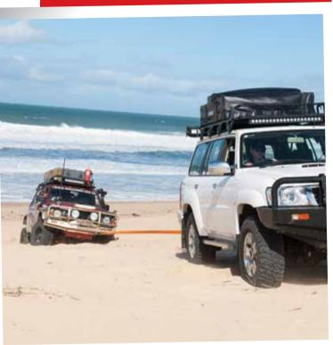
Okay, so the gentle tug didn't work, and you need a decent snatch recovery. Back up the recovering vehicle so there's a decent amount of slack in the strap, and then position the strap with an S up near the recovering vehicle. That way, the person in the vehicle being recovered can watch as the strap takes up tension, and you can ensure that it's not going to knot
