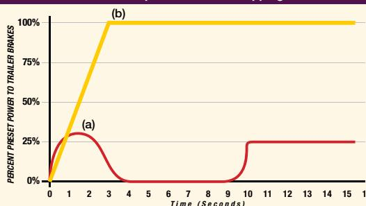
(a) *Proportional controls stop trailers at lower speeds by applying only the amount of power required to gradually slow the trailer at the same rate as the tow vehicle.*
