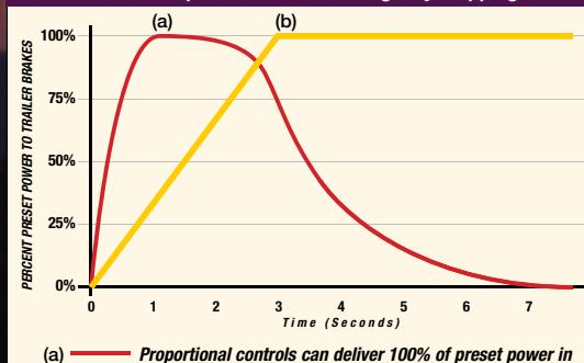
(a) *Proportional controls can deliver 100% of preset power in less than a second.*
